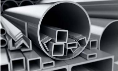
Stainless steel profile is a kind of stainless steel materials with different cross section shape through hot melt and extrusion of stainless steel rods. The production process of stainless steel section mainly includes casting, extrusion and coloring. Furthermore, coloring process contains oxidation, electrophoresis coating, fluorine carbon spraying, powder coating and wooden transfer etc.
